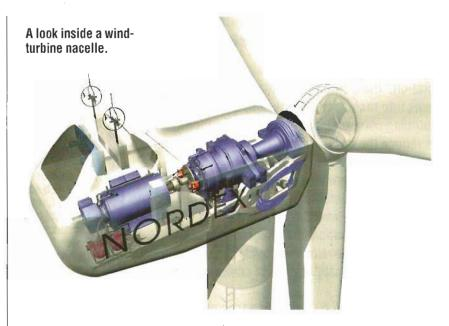
and electrical cables run from the nacelle to the ground. The nacelle contains primary components such as the main axle, gearbox, generator, transformer, control system, and electrical cabinet. The rotor consists of a hub, usually with three blades attached.
