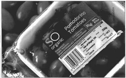
Films such as NatureFlex NVS from Innovia Films in the U.K. are said to provide improved dimensional stability under chill conditions and enhanced transparency in packaging applications. The high-gloss film also has good antistatic properties, is semipermeable to moisture, and will completely biodegrade in a compost heap.
