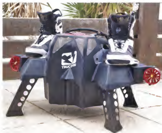
Flyboard Air. Note the fixed boots which keep the pilot attached to the aircraft. Also visible are the two outboard jet engines. Not visible are the four internal jet engines.
