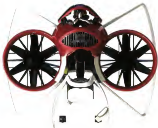
View of the Martin Jetpack from above showing arrangement of the ducted fans.
