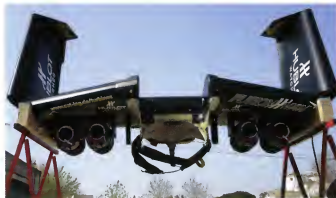
Jetman's jet powered wing in a folded state for transport and also so he can get into helicopters prior to launch.
