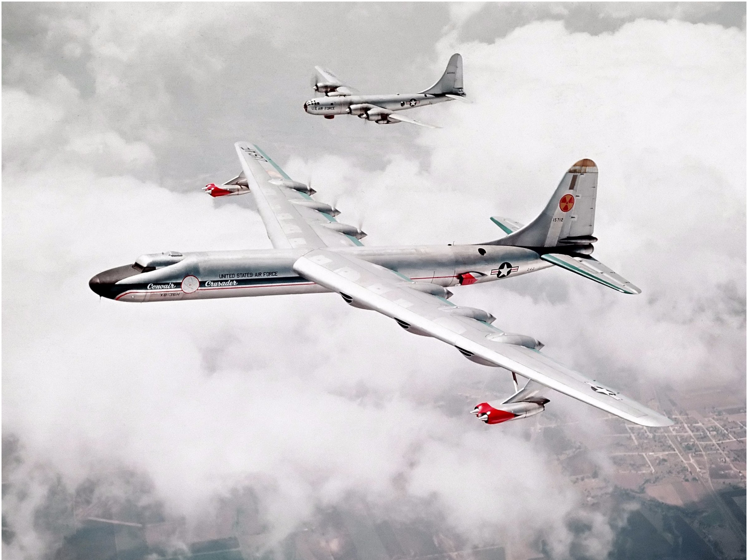
The NB-36H, a jet bomber that flew a nuclear reactor from 1955 through 1957.
