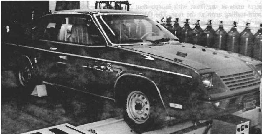
Omnia Research Corporation selected a front-drive Plymouth Horizon TC3 coupe as the mule for its SLX process prove-out. It's shown here on the Omnia chassis dynamometer rollers with the 3-chamber hydrogen generator taking up most of the back seat cargo area. Production unit could be smaller.
