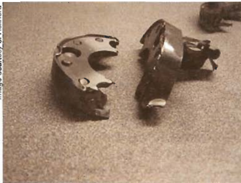
This high speed coupling (several thousand rpm) exceeded its design speed by a substantial amount and burst apart, but was properly captured inside a concrete bunker.
