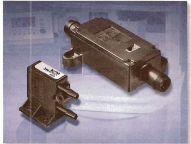
1. Omron's 1-LPM D6F-P series of gas-flow sensors targets medical applications. They're available with bidirectional and unidirectional flow calibrations, with a negative flow indication on the unidirectional version.
