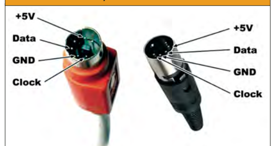
Figure 1. The PS/2 and five pin DIN keyboard connectors.
