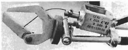
FIG. 15—ASSEMBLED CLAW-TYPE end-effector. Piano wire may be used to connect solenoid and lower portion of claw.
