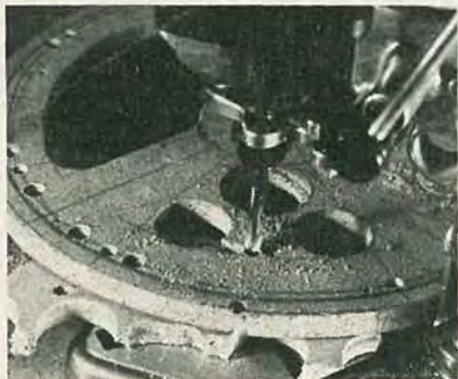
FIG. 29—A SERIES OF SMALL HOLES can be drilled to rough-cut bulkheads to shape.
