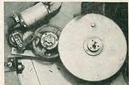
FIG. 32—COMPARE complexity of this speed-reduction train with drive shown below.
