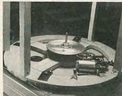
COMPLEX GEAR TRAIN used to slow 10,000-RPM motor to 11-RPM for body rotation.
