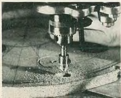
FIG. 30—COUNTERSINKING holes in the bulkhead prevents screwheads from protruding.
