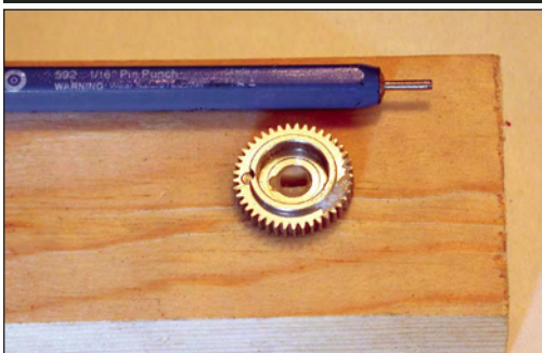
Figure 8. You will need to use a 1/16th-inch diameter pin punch.
