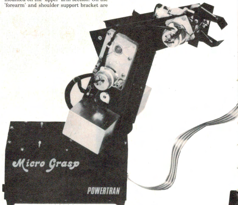
Figure 1. View of the wrist and gripper, showing the various components.
