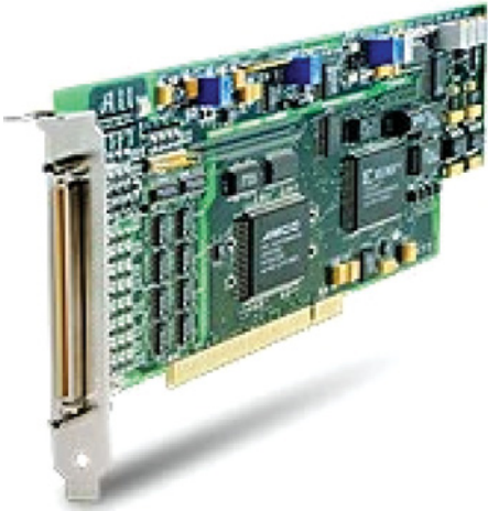
FIGURE 5.57: A commercially available data acquisition board for a PC bus (Model-KPCI-1801HC by Keithley). I/O capabilities are 12-bit 32-Ch differential ended or 64-Ch single ended analog input (multiplexed A/D converter), 12-bit 2-Ch D/A converter, 4-Ch digital input, 8-Ch digital output, maximum sample rate is 333 kHz. Reproduced with permission from Keithley Instruments, Inc.
