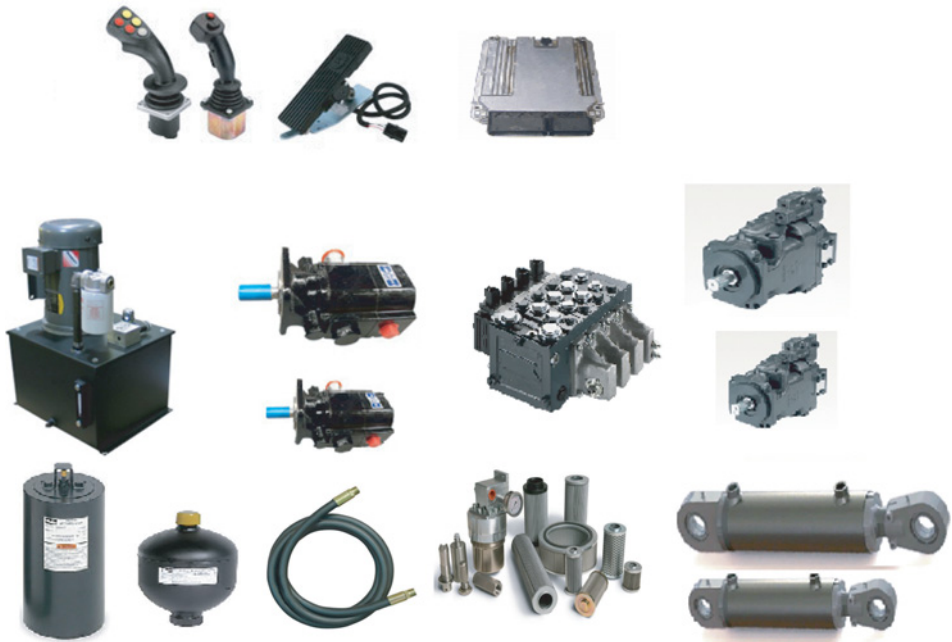
FIGURE 7.1: Components of an electrohydraulic control system: input devices (joysticks), electronic control module (ECM), hydraulic tank, accumulators, pumps, motors, cylinders, valves, hoses and filters. Reproduced with permission from Parker Hannifin.
