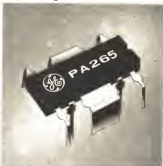
View of I.C. showing unusual heatsink tabs and staggered leads.
