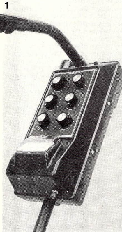
Photo 1. The handle and case assembly of the metal detector showing the high standard of the finished project.
