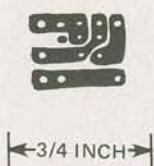
FIG. 10—THE TINY foil pattern shown here is for board 6, the small sensor board.
