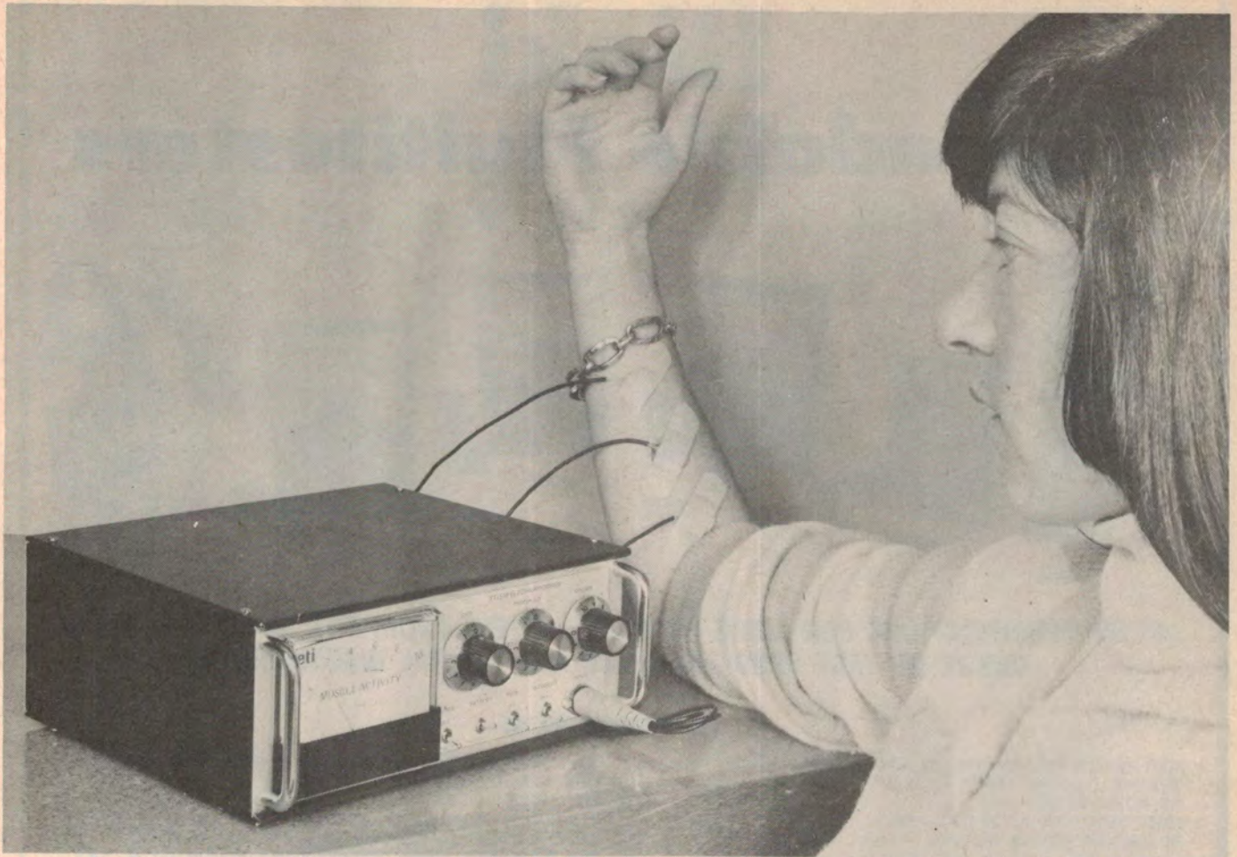
Illustrating muscle relaxation training using our own electromyogram project (see page 35). This project design is based on criteria given by the author of this article and compares very well with commercially made machines. Learning to relax is Jan Collins, our general secretary and office organizer. . . . note calm expression, unfurrowed brow and general aura of peace!
