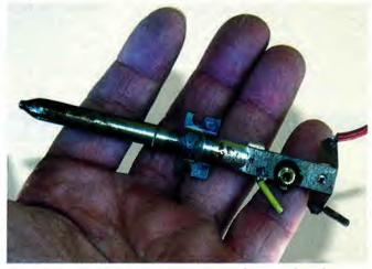
Electric frypan thermostats use a stainless steel probe that can be inserted through the wall of a pipe or into liquids. They can be adjusted to trip at temperatures from about 40-200°C.
