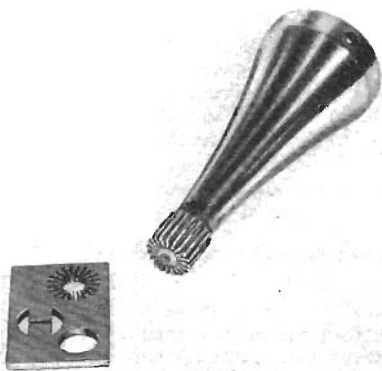
Fig. 4—Sample of complicated machining on tungsten carbide, and tool used.
