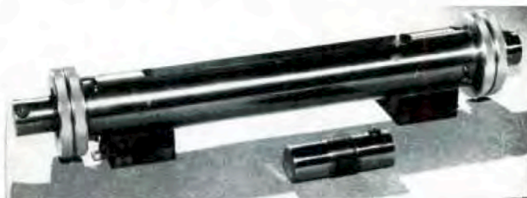
Test chamber used with two transducers for experiments with transmission through various media. One of the transducers of Fig. 1 is shown separately.
