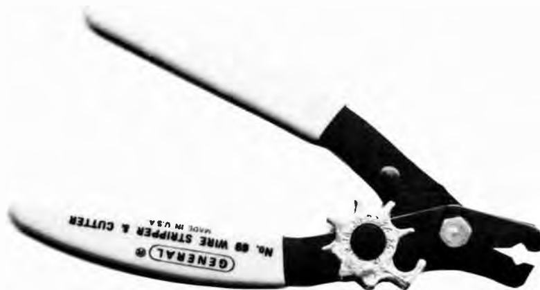
Fig. 5—A handy tool for stripping and cutting hook-up wire and reducing kit-building frustrations.
