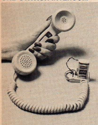
FIG. 1—ONE-STATION INTERCOM is powered by a 9-volt transistor battery and has an LED status indicator.
