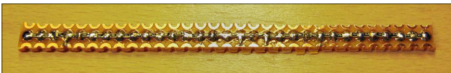
Figure 10. Voltage divider made up of 30 \times 10 M \Omega and a 100 k \Omega precision resistor in the center.
