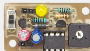
Figure 3. This single-sided circuit board for the marten repeller is available from the Elektor Store.
