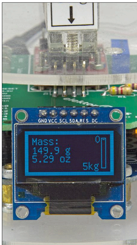
Figure 4. The OLED display shows the weight in grams and ounces, together with a bar graph.
