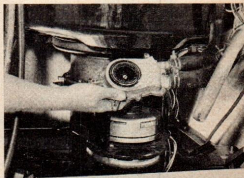
Pump coupling on a General Electric washer must be removed to service the pump or clutch, or to replace the belt. Use hose-clamp pliers to remove the large spring-type clamps that retain the coupling.
