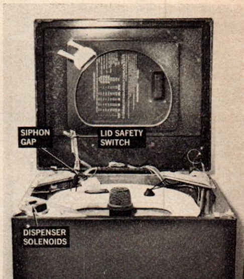
Hinged tops on most newer automatics allow easy access to many components. The inlet valve, snubber or friction pad, lid switch, and many terminals in the wiring harness are serviceable from above.
