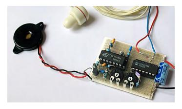
Regardless of volume, this circuit itself can handle the full bat sound spectrum. The only limiting factor is the microphone, for which Thomas 'misused' a so-called 'piezo-conetweeter'; a piezoelectric hightone loudspeaker with a cone shaped membrane (as shown in the picture). A similar loudspeaker can pick up sound waves with frequencies up to 50 kHz, which is adequate to detect most species of bats.
