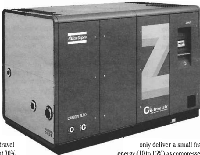
Atlas Copco's Carbon Zero ZR Series of water-cooled, oil-free air compressors typically recover more than 90% of the electrical power needed for compression as hot water.
