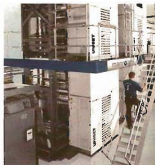
A large German printing-press manufacturer used MathWorks tools for model-based design to develop, test, and implement an efficient, production-ready control system for the cut registers of this state-of-the-art printing press. Engineers developed a Simulink model of the control system based on a proportional integral derivative (PID) controller. Open-loop testing of several strategies identified the one resulting in the most efficient device.
