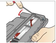
7 The soleplate wheels or axles can be prised out from the soleplate assembly if necessary using a thin, flat bladed screwdriver. To fit, firmly press both parts into the soleplate assembly.
