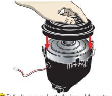
30 Fit the fancase seal onto the base of the motor.
