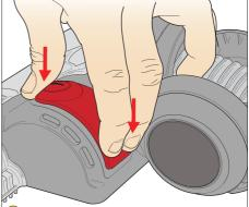
Decate the front of the brushbar actuator into the top of the brushbar motor cover. Then force the rear of the actuator into the cover. Turn the floor tool over and locate the lip of the actuator over the ledge in the underside of the brushbar motor cover.
