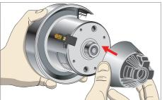
27 Fit the motor mount onto the motor plate. Locate the motor plate onto the motor.
