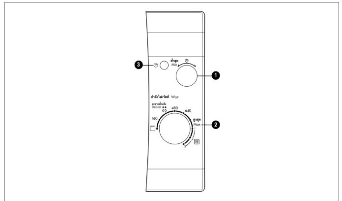
TIMER / WEIGHT SELECTOR CONTROL: Used to set the cooking time.
