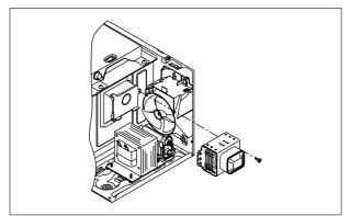
**CAUTION**: Never install the magnetron without the metallic gasket plate which is packed with each magnetron to prevent microwave leakage. Whenever repair work is carried out on magnetron, check the microwave leakage. It shall not exceed 4mW/cm² for a fully assembled oven with door normally closed.
