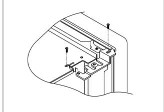
**NOTE**: After replacing the door assembly, perform a check of correct alignment with the hinge and cavity front plate.
