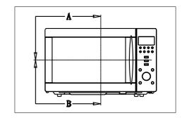
NOTE: A small gap may be acceptable if the microwave leakage does not exceed 4mW does not exceed 4mW/cm².
