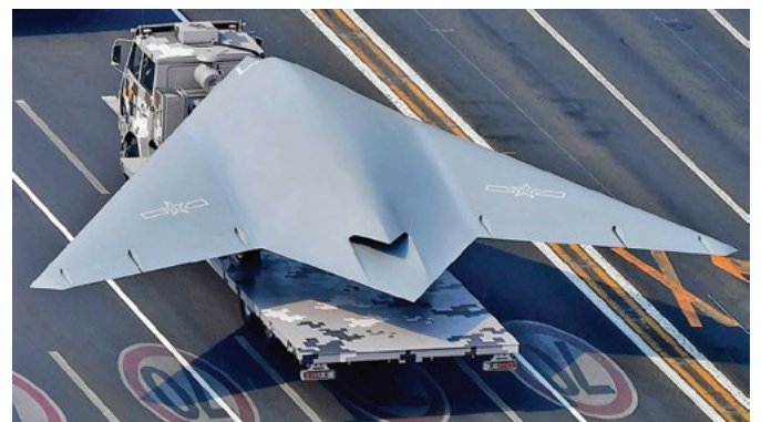
Fig.27: a Chinese GJ-11 Unmanned Combat Aerial Vehicle showing various stealth characteristics, including a shrouded exhaust to minimise infrared signature, blended wings, smooth shape, low overall profile and a flying wing design with no fuselage or tail fins. The result is a low radar signature. It has been suggested that this is not a real flying aircraft but a mockup.
