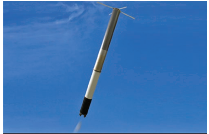
Fig.22: the Australian-developed Nulka decoy; Australia's largest defence export, worth $1 billion in export revenue. It is more effective if the radar signature of the ship it is protecting is minimised, so the Nulka presents a larger target.
