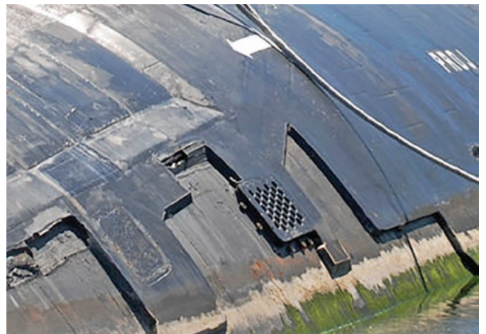
Fig.30: acoustic tiles on a modern submarine; some that have fallen off due to defective adhesion. There is also what appears to be a vent. Adhesion of tiles to the hull is a problem; the tiles are relatively thick, heavy and expensive. Research aims to minimise these characteristics.
