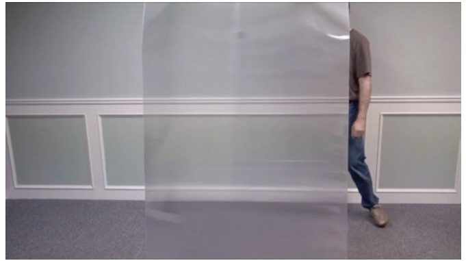
Fig.32: a demonstration of the HyperStealth Quantum Stealth technology. Despite the name, there is no quantum mechanical effect involved.
