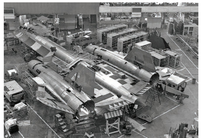
Fig.4: an SR-71 Blackbird under construction, showing the wedges in the wing trailing edges (from siliconchip.com.au/link/aaza ).
