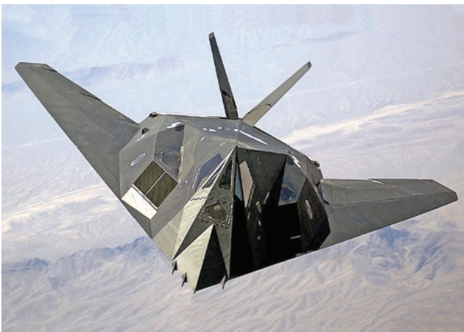
Fig.7: the US F-117A flew from 1981 to 2008. It was the first purpose-built production stealth aircraft, designed to have a low radar and infrared signature.
