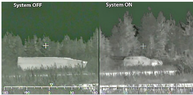
Fig.28: Adaptiv infrared stealth technology on an armoured vehicle with the system off and on. Panels are heated or cooled to give the appearance of a car when viewed with infrared imaging equipment.
