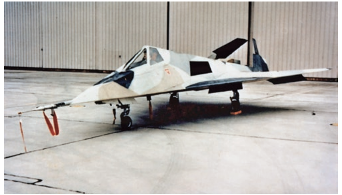
Fig.6: the Lockheed “Have Blue” HB1001 proof-of-concept stealth technology demonstrator. It was developed into the F-117A Nighthawk which first flew in 1977 and was the first aircraft whose shape was specifically designed to minimise radar cross-section. Two prototypes were built; both crashed, but the stealth concept was proven.
