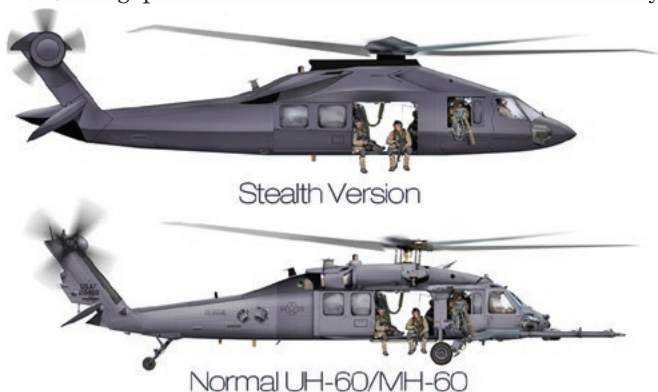
Fig.20: a comparison of a standard Black Hawk helicopter (as used by Australia) and the stealth version, which has an extra rear rotor blade, and the main rotor has downturned tips. The stealth version is also much smoother, with fewer protuberances, plus angled sides which are likely made of or coated with radar absorbing materials.
