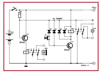
is shown on the left in the circuit diagram. It consists of a relay (K2), a pull-up resistor (R1) and a transistor. The relay is used to switch a buzzer or bell. Switch S2 is used to reset the system. The client systems are connected
