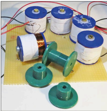
Figure 7. Winding formers made using a 3D printer.
