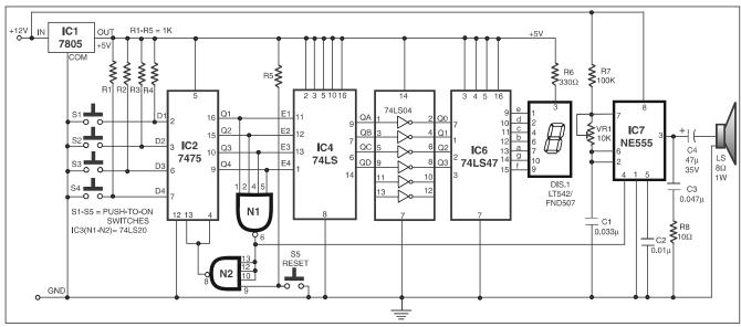
The circuit presented here determines as to which of the four contestants first pressed the button and locks out the remaining three entries. Simultaneously, an audio alarm and the correct decimal number display of the corresponding contestant are activated.
