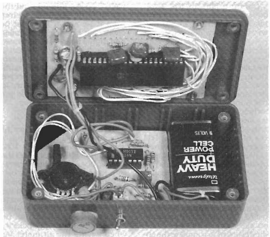
FIG. 6—HERE'S THE AUTHOR'S PROTOTYPE. Notice the four wires that connect the analog and digital boards together.
