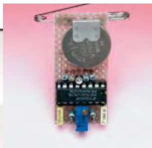
Figure 2. Fit the components as close together as possible on a piece of perforated circuit board to keep the finished circuit compact.
