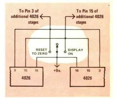
You can use separate display on and reset switches, as shown in the projet diagram, or a single pole, center off, double throw switch as shown above.
