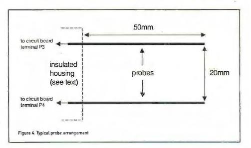
distance apart. The required spacing will change if the length of the probes is significantly different.
