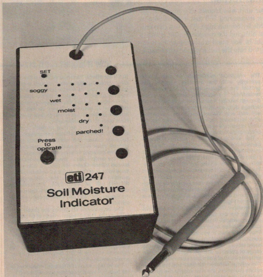
With the probe in 'soggy' soil, only the top LED will light. In 'wet' soil, the top two LEDs will light — and so on until, with the probe in 'parched' soil, all LEDs will light!
