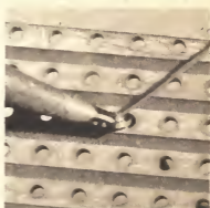
Fig. 13. Allow the solder to flow evenly over copper and wire
