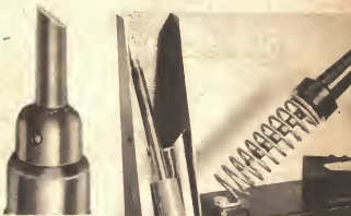
Fig. 2. The tip must be flat and tinned
