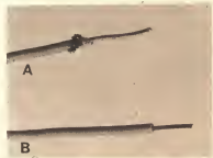
Fig. 6. (a) Stripped insulation by hot iron (bad) and (b) with strippers (good)
