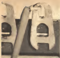
Fig. 8. Tinned clean tags and wire fitted
