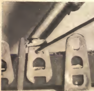
Fig. 9. Apply iron to tag and wire, then the solder
