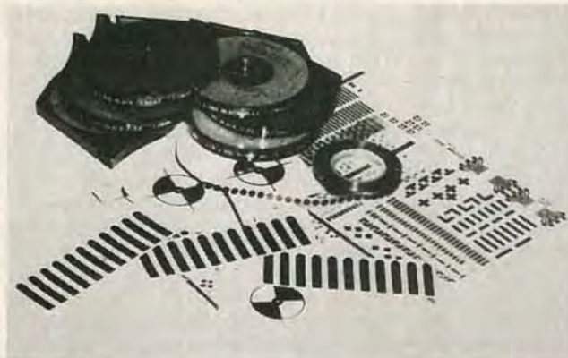
FIG. 3—DRAFTING AIDS, such as the ones shown here, can be very useful in completing your layout.
