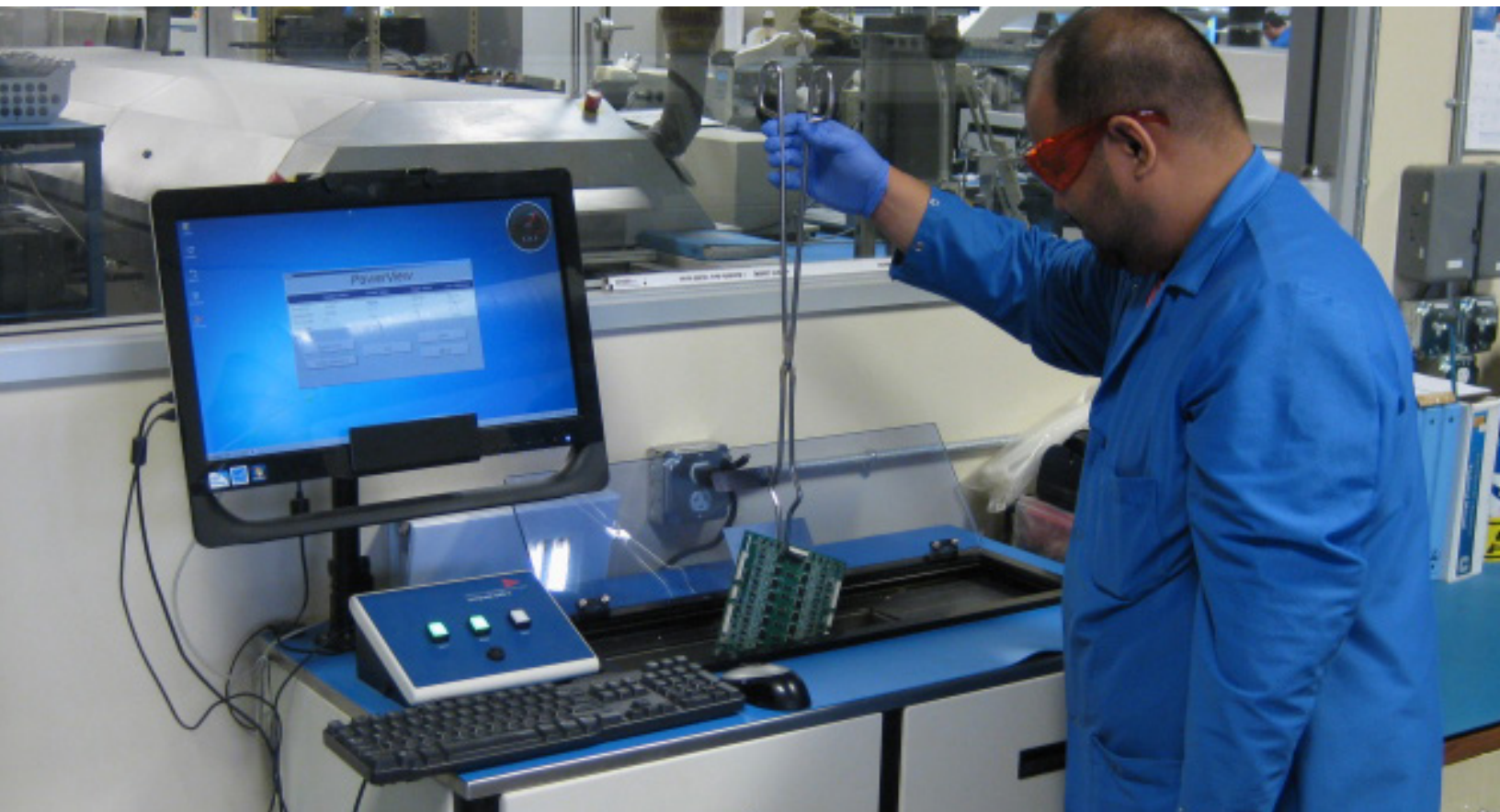
Fig. 1. Ionograph tester for checking ionic contamination after batch cleaning is finished.
