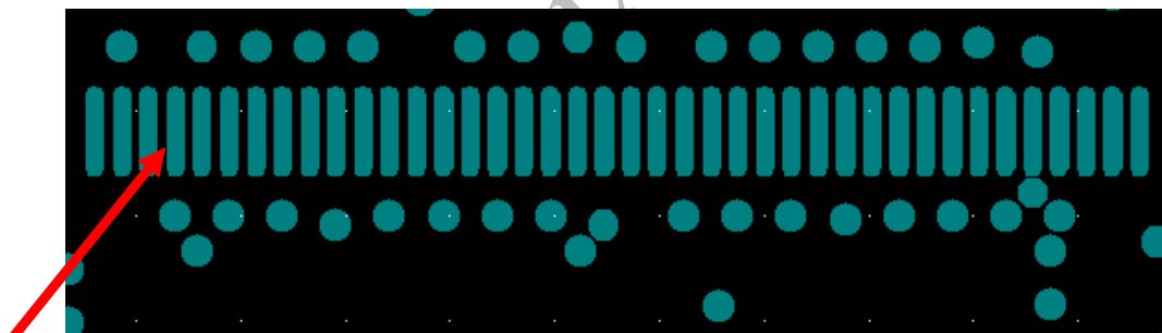
Fig 12 Solder Mask layers of Fig 11
