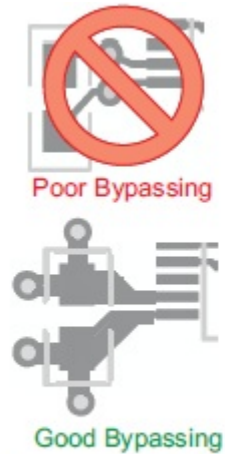
Figure 12. Poor and Good Placement and Routing of Bypass Capacitors
