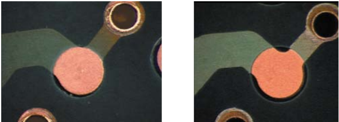
Figure 12: Top View of land illustrating increase of effective land diameter due to trace connections
