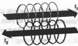
Figure 2 Magnetic fields from the outgoing current (red) nearly cancel the equal-but-opposite magnetic fields from the returning signal current.
