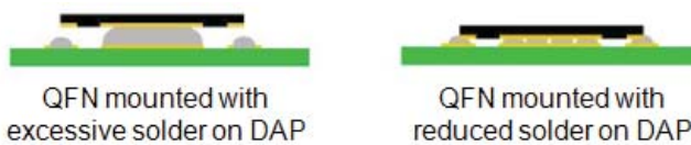
Figure 9: Excessive thermal pad paste mask on the Die Attach Pad
