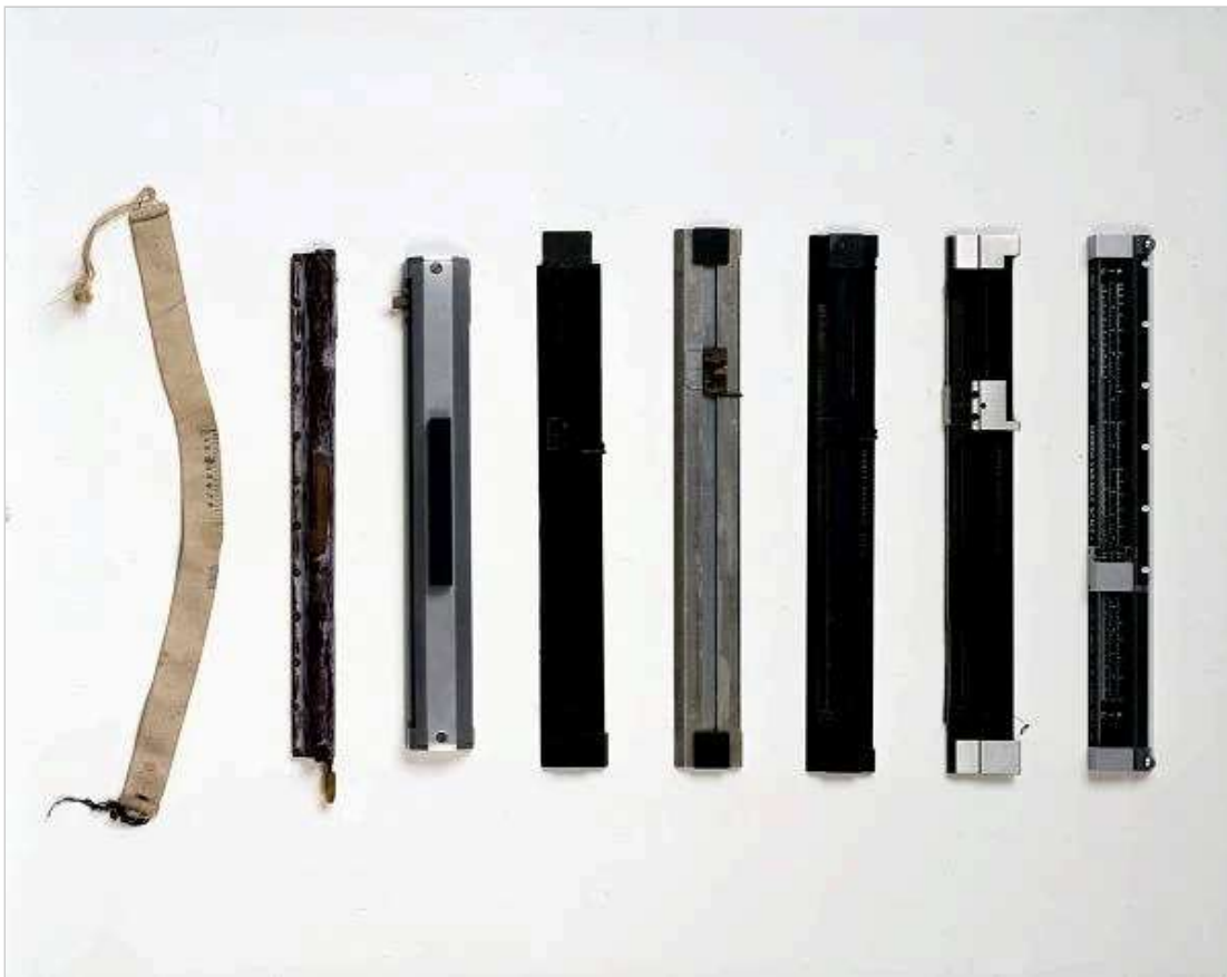
Prototypes and versions of the Gerber Variable Scale. Image used courtesy of the National Museum of American History .
